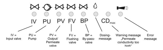
The LEDs display active plant components and occurring error messages.
